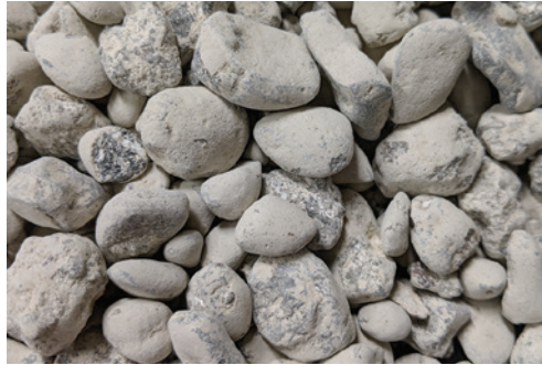
Recycled concrete particles are coated with synthetic limestone, forming a coating that is 44% by mass CO 2 . Photos: Blue Planet Ltd.
