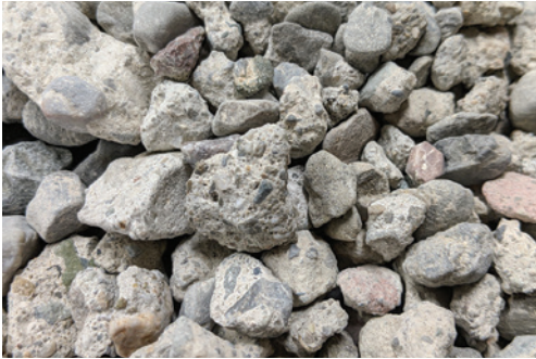
Recycled concrete particles are coated with synthetic limestone, forming a coating that is 44% by mass CO 2 . Photos: Blue Planet Ltd.
